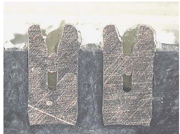
Insulation Displacement Contact of core wire
