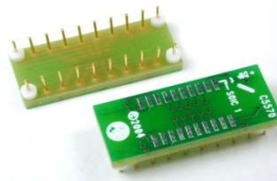
SOIC to DIP convertor using blind hole technology
