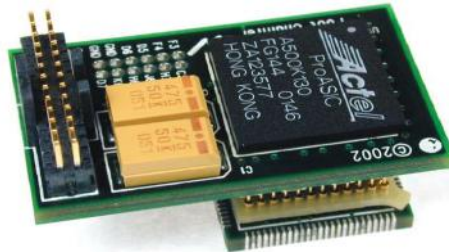
Daughter card module Interfaced to QFP footprint
