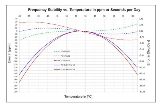
It can easily be seen that high and low temperatures cause comparatively large frequency deviations in tuning fork crystals (solid lines). The curves of oscillators using AT-cut quartz blanks (dashed lines), however, show much smaller errors.
