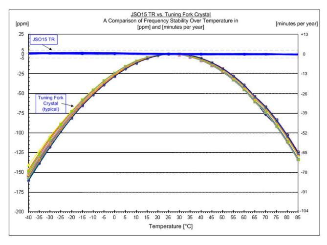
The bottom line is: 32.768 kHz oscillators have some major advantages compared to classic tuning fork crystals: They are easier to use and – depending on the model – much more accurate than the classic tuning fork crystals due to temperature compensation and the use of an AT-cut quartz blank. However, tuning fork crystals are still in need: In properly designed circuits, they also ensure stable frequencies.
