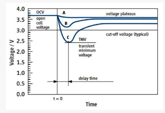
The diagram shows the effects of passivation as a function of the required discharge currents. Low or medium discharge currents as depicted by curves A and B would thus not have a great effect on the battery as the operating voltage will drop only slightly before returning to ist normal level.
