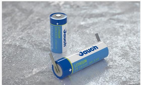
Lithium thionyl chloride (LiSOCl<sub>2</sub>) batteries are special in many ways; with 3.6 volts, they have the highest cell voltage of any primary batteries available. They are also extremely durable and can be safely stored for long periods of time. This excellent shelf life is the result of another special feature of LiSOCl<sub>2</sub> batteries called "passivation".
