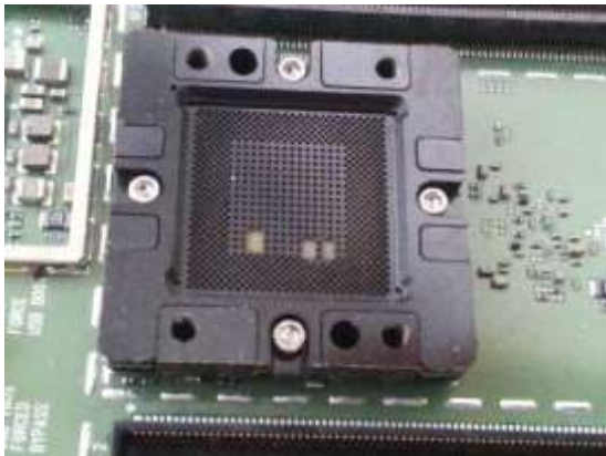
Above Near Zero Footprint Spring Pin Socket mounted to an evaluation board
