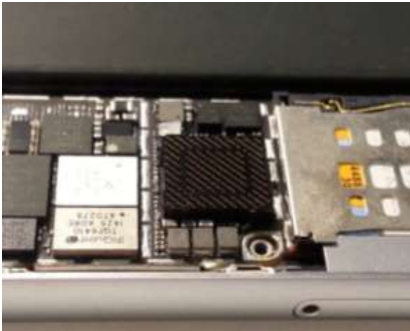
Above Grypper installed into a phone – Grypper socket is the same size as the device so it fits into the exact space as the device
