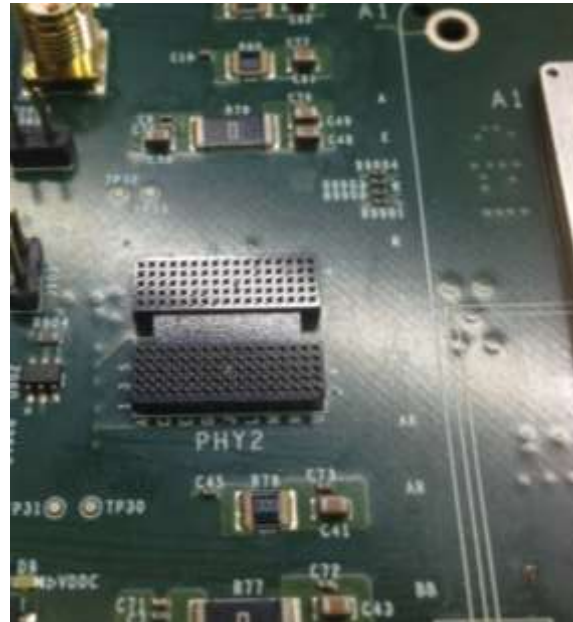
Above Grypper on a validation PCB for GDDR5 Device
