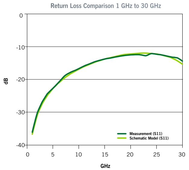
Figure 9. GSG P2A Return Loss, 0.8 pitch
