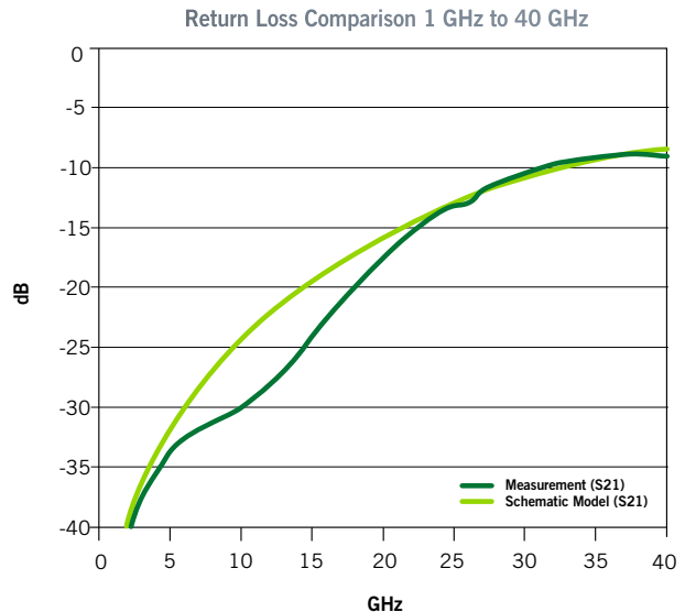
Figure 16. GSG P8A Return Loss, 0.8 pitch
