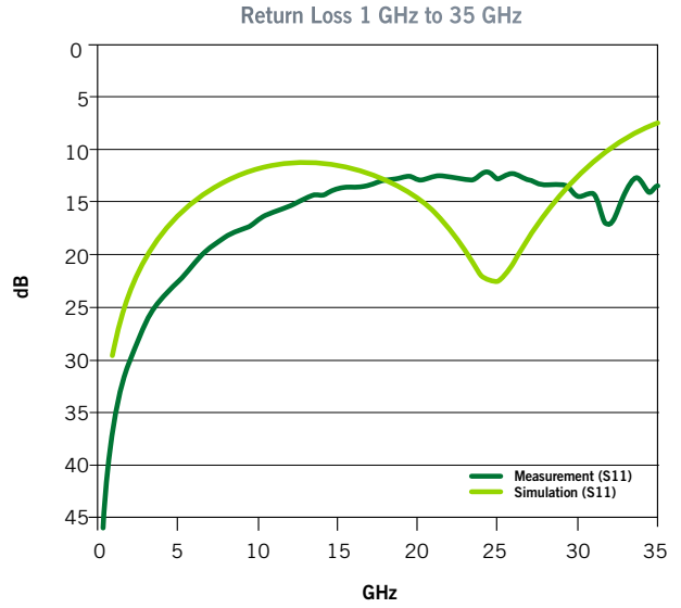
Figure 5. GSG P2A Return Loss comparison, 0.8 mm pitch
