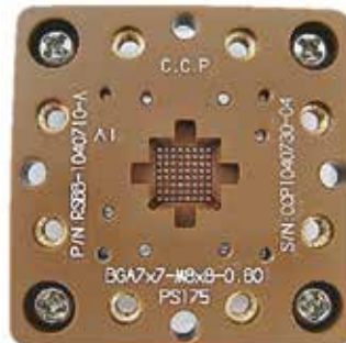
BGA Socket Pitch 0.8mm
