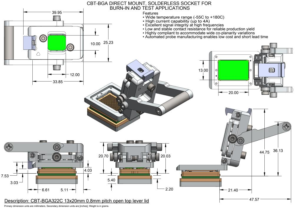
Tolerances: Hole diameters ±0.03mm [±0.001"], Pitches (from true position) ±0.025mm [±0.001"], substrate thickness tolerance ±10%, all other tolerances ±0.13mm [±0.005"] unless stated otherwise. Materials and specifications are subject to change without notice.
