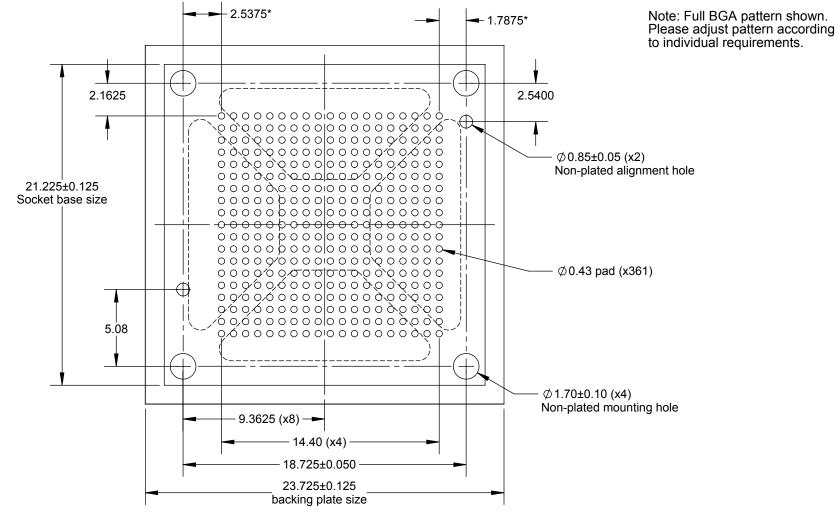
Target PCB Recommendations Total thickness: 1.6mm min.
