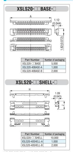
\*XSLS20- $\square$ BASE- $\square$  and XSLS20- $\square$ SHELL- $\square$  are component parts of XSLS20-\\_\\_.
