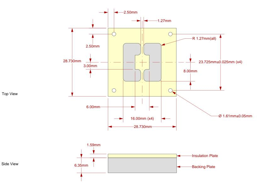
Description: Backing Plate with Insulation Plate
