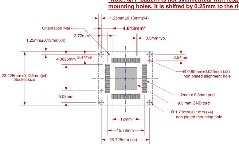
\*Note: QFP pattern is not symmetrical with respect to the mounting holes. It is shifted by 0.25mm to the right.
