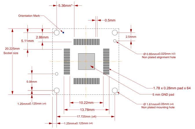
Target PCB Recommendations Total thickness: 1.6mm min. Plating: Gold or Solder finish PCB Pad height: Same or higher than solder mask
