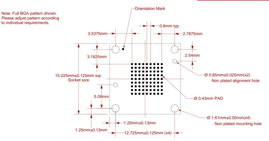
Target PCB Recommendations Total thickness: 1.6mm min. Plating: Gold or Solder finish PCB Pad height: Same or higher than solder mask
