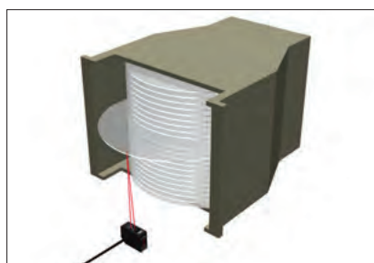
Wafer protrusion detection in cassettes
