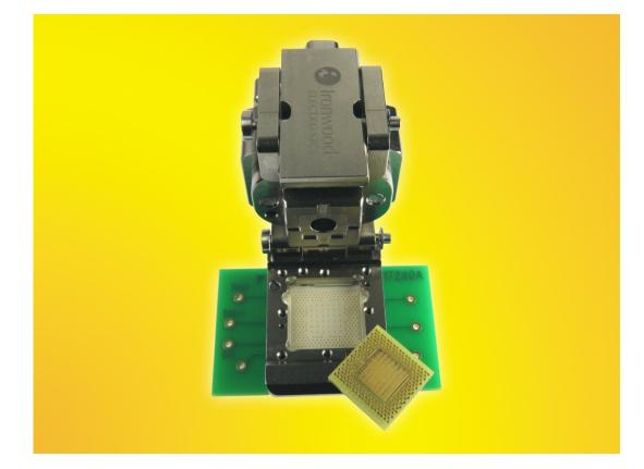
The SS-QFN204A-01 socket utilizes high endurance spring pins, which allow for product use in multiple applications including burn-in, production test, and prototype development. In addition to its wide temperature range and high endurance the pin operates with an inductance of 1.3nH and with a capacitance to ground of 0.53pF. Current carrying capacity is 1.5 amps per pin. Normal force for actuation is only 16gms per pin with a typical contact resistance of 82 mOhms.
