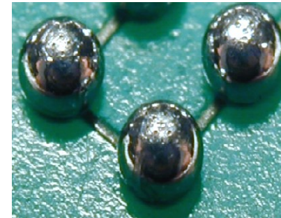
Wire marks on BGA
