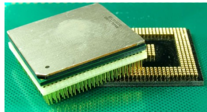
Pluggable adapter pair with soldered device
