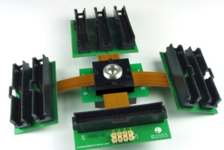
0.5mm pitch 21x21 array 289 position BGA solder balls to AMP 104068 connectors using rigid flex PCB with socket fixture
