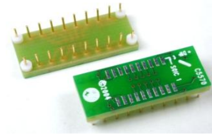
SOIC to DIP converter using blind hole technology
