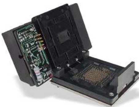
Test and Burn-in Socket with Integrated Heat Sink, Heater, Temperature Sensing RTD, and Programmable Controller
