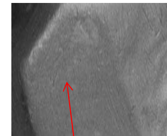
No Sn contamination on pin tip after 500K cycles
