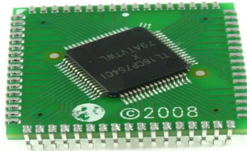
QFP device mounted to PLCC Footprint on target board with shortest trace length
