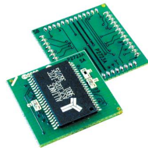
SOIC device mounted to PLCC footprint using solder column technology for high volume production
