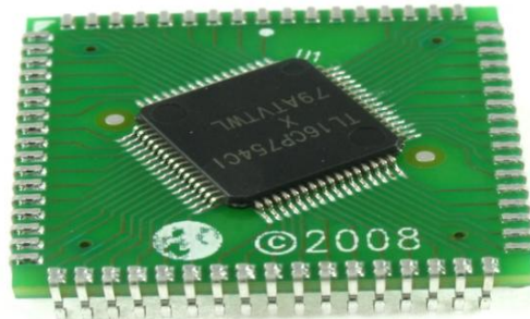
QFP device mounted to PLCC Footprint on target board with shortest trace length
