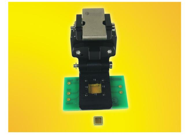
The CG25-QFN-2003 sockets are constructed with high performance and low inductance elastomer contactor. The temperature range is -35C to +100 C. The pin self inductance is 0.06 nH and mutual inductance of 0.019 nH. Capacitance to ground is 0.129 pF and mutual capacitance is 0.017pF. Current capacity is 2 amps per pin.
