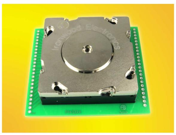
The SG-BGA-6450 socket is constructed with high performance and low inductance elastomer contactor. The temperature range is -35°C to +100°C. The pin self inductance is 0.15 nH and mutual inductance of 0.025 nH. Capacitance to ground is 0.01 pF. Current capacity is 2 amps per pin. Works with Xilinx FPGA's such as 2104BGA, 47.5mm square package with 46x46 array and 1mm pitch.
