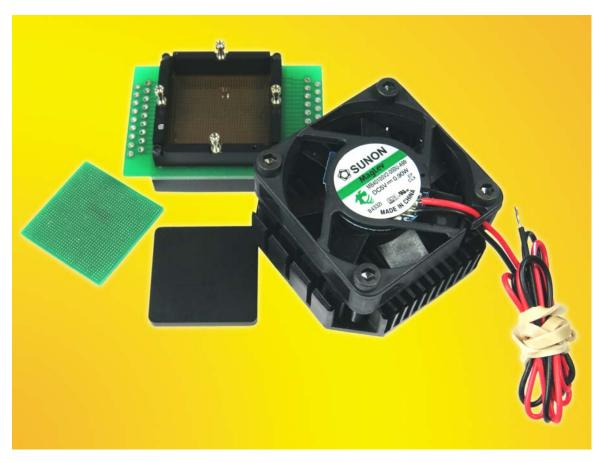
The SG-BGA-9002 sockets are constructed with high performance and low inductance elastomer contactor. The temperature range is -35C to +100 C. The pin self inductance is 0.118 nH and mutual inductance of 0.025 nH. Capacitance to ground is 0.229 pF and mutual capacitance is 0.025pF. Current capacity is 2 amps per pin.
