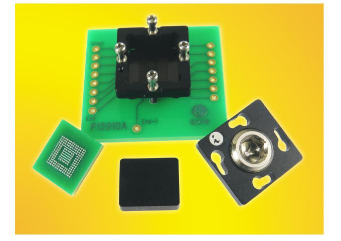
The SG-BGA-7292 sockets are constructed with high performance and low inductance elastomer contactor. The temperature range is -35 °C to +100 °C. The pin self inductance is 0.15 nH and mutual inductance of 0.025 nH. Capacitance to ground is 0.01 pF. Current capacity is 2 amps per pin. Works with IC's such as Kingston eMMC BGA153, 13x11.5mm with 0.5mm pitch and 14x14 ball array.
