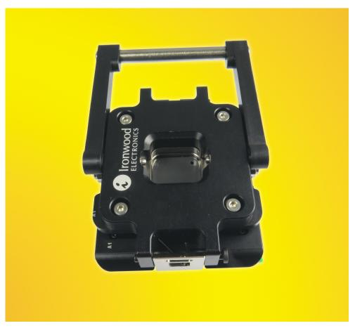
The CG-BGA-4022 sockets are constructed with high performance and low inductance elastomer contactor. The temperature range is -35 C to +100 C. The pin self inductance is 0.11 nH and mutual inductance of 0.028 nH. Capacitance to ground is 0.028 pF. Current capacity is 2 amps per pin.
