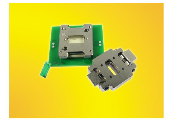
This socket can be used for quick device screening, device characterization at extreme temperatures as well as final production test.
