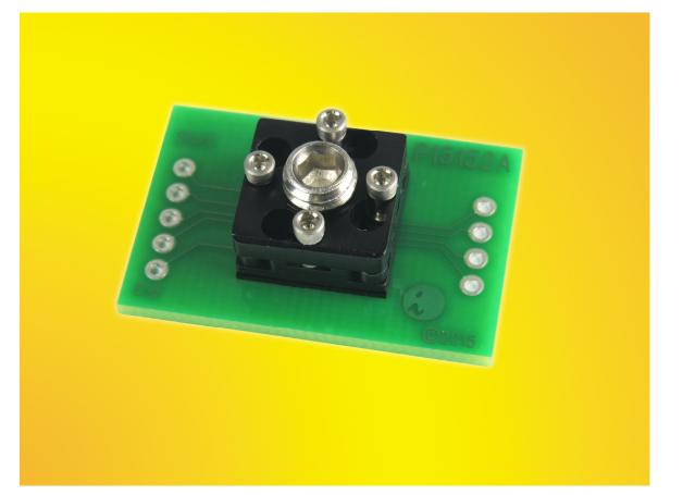
The SG25-BGA-2016 sockets are constructed with high performance and low inductance elastomer contactor. The temperature range is -35C to +100 C. The pin self inductance is 0.06 nH and mutual inductance of 0.019 nH. Capacitance to ground is 0.129 pF and mutual capacitance is 0.017pF. Current capacity is 2 amps per pin.
