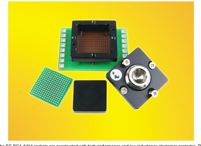
The SG-BGA-6434 sockets are constructed with high performance and low inductance elastomer contactor. The temperature range is -35 °C to +100 °C. The pin self inductance is 0.11 nH and mutual inductance of 0.028 nH. Capacitance to ground is 0.028 pF. Current capacity is 2 amps per pin.
