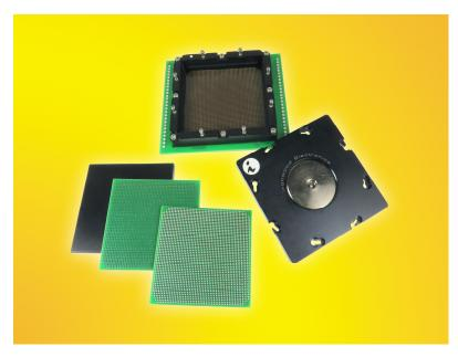
The SG-BGA-6422 socket is constructed with high performance and low inductance <u>elastomer contactor</u>. The temperature range is -35 °C to +100 °C. The pin self inductance is 0.15 nH and mutual inductance of 0.025 nH. Capacitance to ground is 0.01 pF. Current capacity is 2 amps per pin. Works with IC's such as Xilinx BGA, 52.5mm square package with 51x51 array and 1mm pitch.
