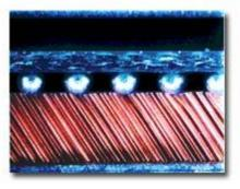
This insulation plate sandwiches between the backing plate and target PCB. The sockets have a precision design, which guides the IC to the exact position for connection of each ball and uses an aluminium heat sink screw to provide compressive force. The sockets are designed to dissipate up to several watts without extra heat sinking and can handle up to 100 watts with a custom heat sink. The user simply places the IC into the socket, places the compression plate, swivels the lid, and
