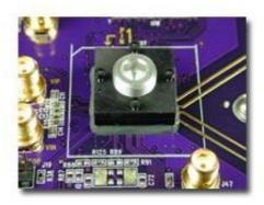
If through-holes are unacceptable, or if <2.5mm keep out zone is required, an epoxy mounting option may be considered. While this creates a more or less permanent bonding of the socket to the PC Board, the socket is designed such that the contacting elements are replaceable should damage or excessive wear occur. These patented ZIF sockets are simply mounted to the target PCB by an epoxy band around the perimeter. The socket is placed into position
