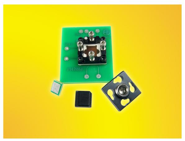
The SG-MLF-7084 sockets are constructed with high performance and low inductance elastomer contactor. The temperature range is -35C to +100 C. The pin self inductance is 0.118 nH and mutual inductance of 0.025 nH. Capacitance to ground is 0.229 pF and mutual capacitance is 0.025pF. Current capacity is 2 amps per pin.
