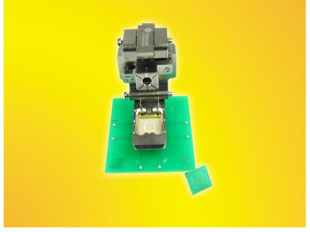
This socket can be used for quick device screening, device characterization at extreme temperatures as well as final production test.
