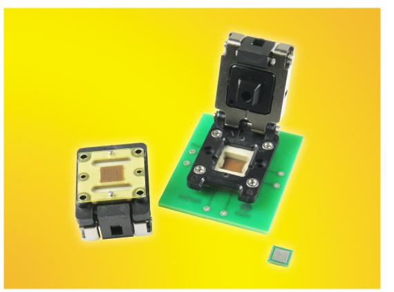
The CG-QFN-7009 sockets are constructed with high performance and low inductance elastomer contactor. The temperature range is -35 C to +100 C. The pin self inductance is 0.11 nH and mutual inductance of 0.028 nH. Capacitance to ground is 0.028 pF. Current capacity is 2 amps per pin.
