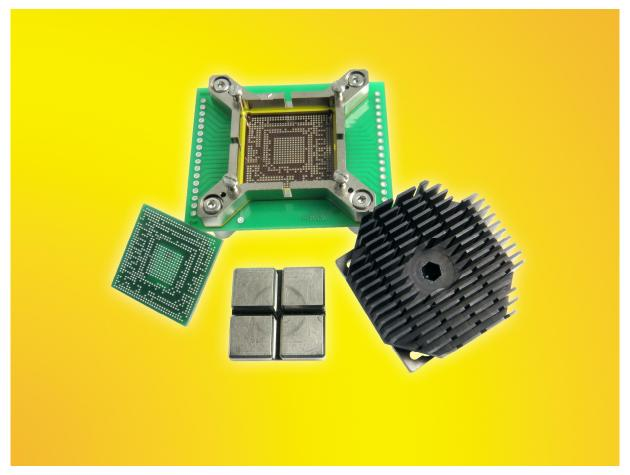
The GT-BGA-6008 socket is constructed with high performance and low inductance elastomer contactor. The temperature range is -55 C to +160 C. Works with IC's such as BGA, 27x27mm with 32x32 array and 0.8mm pitch.
