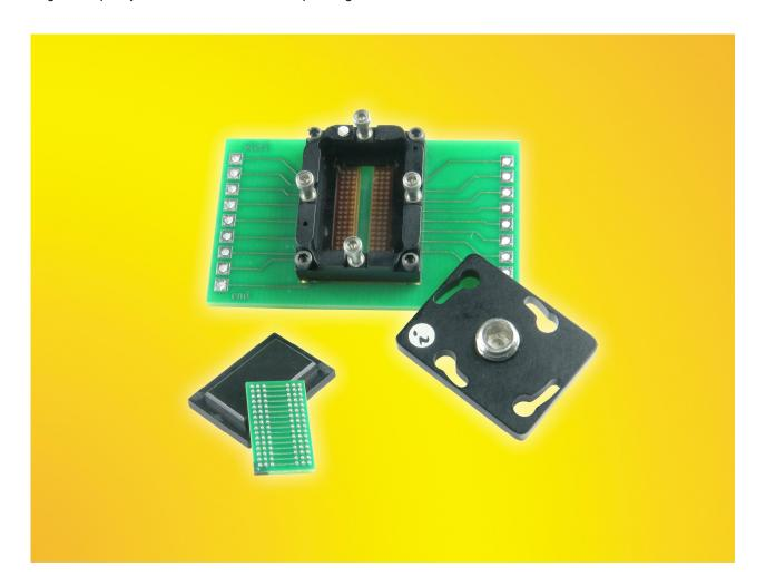
The SG-BGA-6410 socket is constructed with high performance and low inductance elastomer contactor. The temperature range is -35 C to +100 C. The pin self inductance is 0.15 nH and mutual inductance of 0.025 nH. Capacitance to ground is 0.01 pF. Current capacity is 2 amps per pin. Works with IC's such as Hynix, Micron, Winbond DDR3 SDRAMs in BGA package with 16x9 array and 0.8mm pitch.
