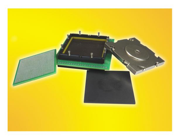
The SG-BGA-6409 socket is constructed with high performance and low inductance elastomer contactor. The temperature range is -35 C to +100 C. The pin self inductance is 0.15 nH and mutual inductance of 0.025 nH. Capacitance to ground is 0.01 pF. Current capacity is 2 amps per pin. Works with IC's such as Xilinx BGA, both 45mm square and 47.5mm square package with 44x44 array and 1mm pitch.
