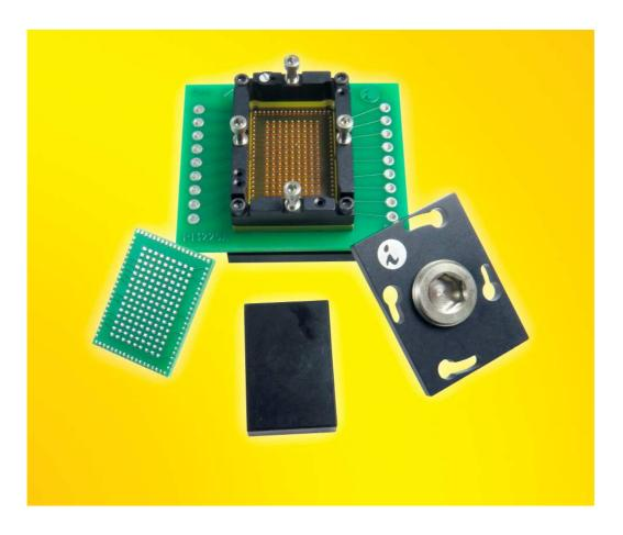
The SM-QFN-9019 socket is constructed with high performance and low inductance elastomer contactor. The temperature range is -55 C to +150 C. The pin self inductance is 0.10 nH and mutual inductance of 0.007 nH. Capacitance to ground is 0.069 pF. Current capacity is 4 amps per pin.
