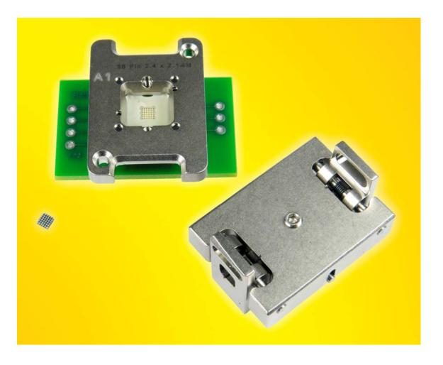
The socket is mounted using supplied hardware on the target PCB with no soldering. To use, place the BGA device into the socket base and lock the double latch socket lid on to the base using the latch. The socket uses a compression wave spring to apply constant downward pressure enabling the device be interconnected to the target PCB. This socket can be used for hand test and quick device screening applications with the most stringent requirements.
