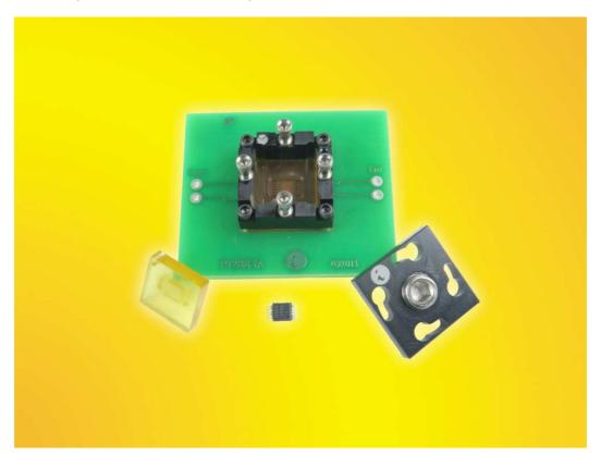
The SG-SOIC-3005 sockets are constructed with high performance and low inductance gold plated <a href="embedded wire on elastomer">embedded wire on elastomer</a> as interconnect material between device and PCB. The temperature range is -35C to +100 C. The pin self inductance is 0.15 nH and mutual inductance of 0.025 nH. Capacitance to ground is 0.01 pF. Current capacity is 2 amps per pin.
