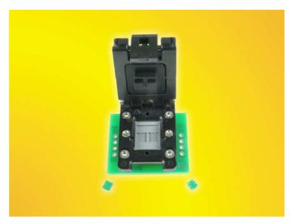
The socket is mounted using supplied hardware on the target PCB with no soldering, and uses the smallest footprint in the industry. The smallest footprint allows inductors, resistors and decoupling capacitors to be placed very close to the device for impedance tuning. To use, place DFN device into the socket and close the lid by snapping to the latch. This socket can be used for quick device screening, device characterization at extreme temperatures as well as final
