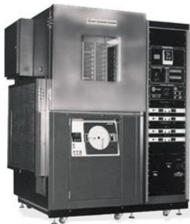
Loranger 85C / 85% Relative Humidity Chamber with Wiring Feed Through, Internal Rack, Equipment Rack, Controls and Power Supplies
