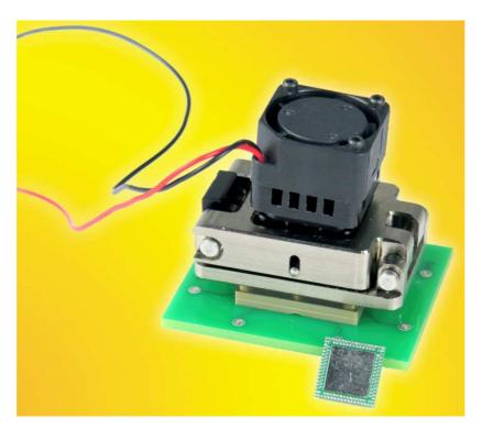
This socket can be used for quick device screening, device characterization at extreme temperatures as well as final production test.
