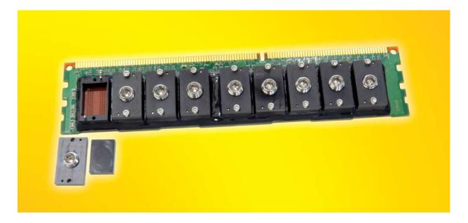
The SG-BGA-6374 sockets are constructed with high performance and low inductance elastomer contactor. The temperature range is -35 C to +100 C. The pin self inductance is 0.11 nH and mutual inductance of 0.028 nH. Capacitance to ground is 0.028 pF. Current capacity is 2 amps per pin. Multiple BGA sockets can be mounted on UDIMM as shown in the picture and can be plugged into mother board for evaluation.
