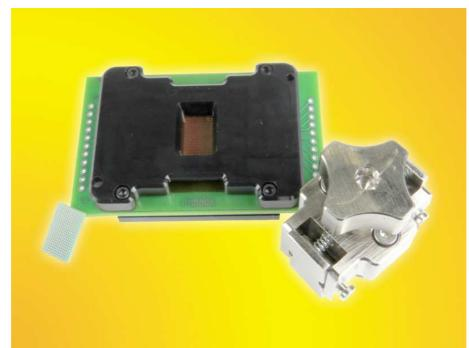
The CG-BGA-5019 sockets are constructed with high performance and low inductance elastomer contactor. The temperature range is -35 C to +100 C. The pin self inductance is 0.11 nH and mutual inductance of 0.028 nH. Capacitance to ground is 0.028 pF. Current capacity is 2 amps per pin.
