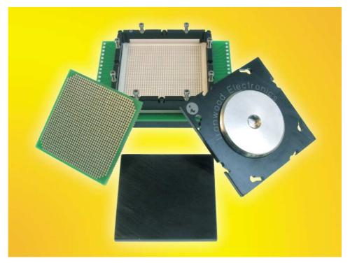
The SG-CGA-7002 socket is constructed with high performance and low inductance <u>elastomer contactor</u>. The temperature range is -35 C to +100 C. The pin self inductance is 0.15 nH and mutual inductance of 0.025 nH. Capacitance to ground is 0.01 pF. Current capacity is 2 amps per pin. Works with IC's such as Actel CCGA, 37.5X37.5mm with 36X36 array and 1mm pitch.
