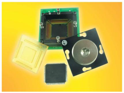
The SG-QFE-7011 sockets are constructed with high performance and low inductance gold plated embedded wire on elastomer as interconnect material between device and PCB. The temperature range is - 35°C to +100°C. The pin self inductance is 0.15 nH and mutual inductance of 0.025 nH. Capacitance to ground is 0.01 pF. Current capacity is 2 amps per pin.
