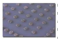
Ironwood Electronics SM/SMP socket uses SM & SMP contact technology for high speed, low inductance, high endurance and wide temperature applications. SM Contact is a unique contact that has precise silver balls held together by a proprietary conductive formulation. These conductive columns (diameter optimized for 50 ohm impedance) are suspended in a
